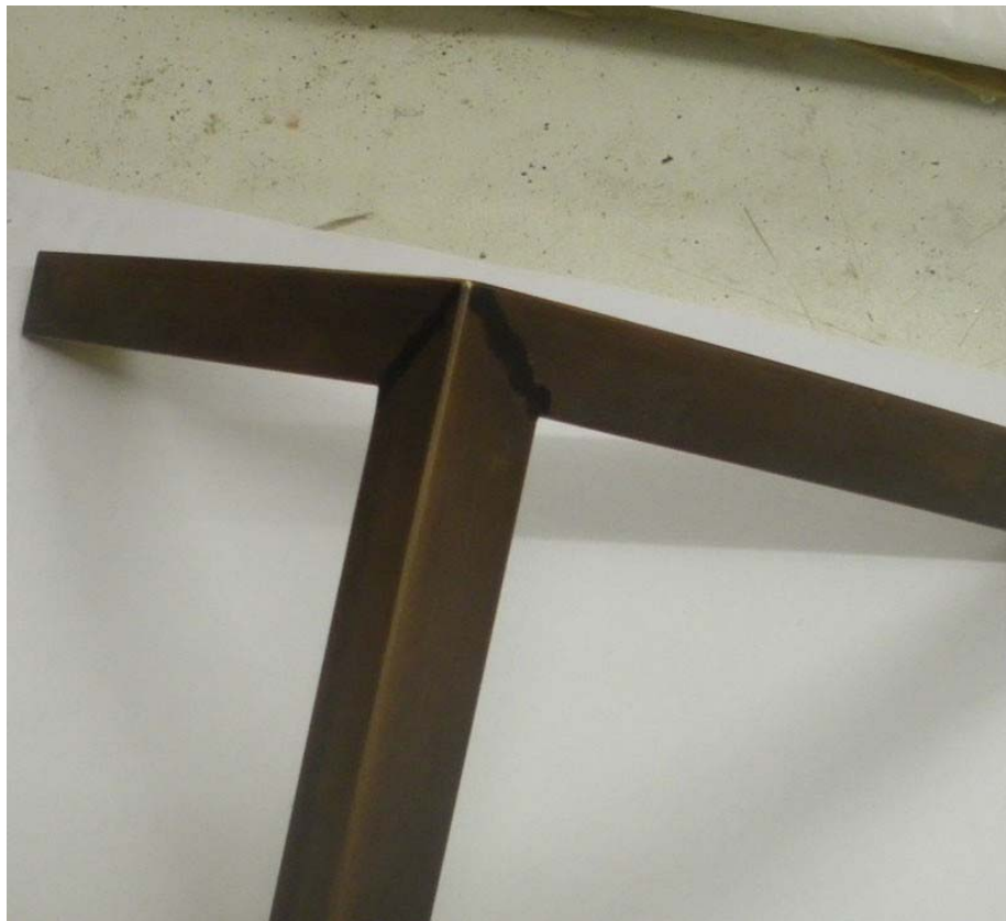
Figure 4: Brass – welded and patinated – crisp edges, fairly strong, but shows the joins
